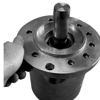
9. Position and carefully press, by hand, the combined flange and swash plate into the housing. IMPORTANT: Ensure not to cut the O-ring.
