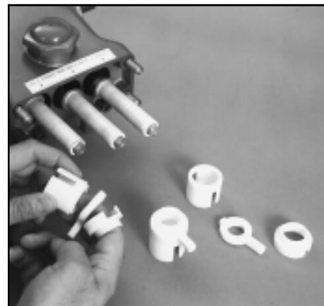
Removal of Seal Retainers and Wicks
