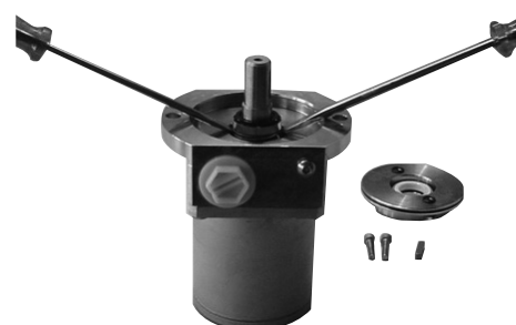
4. Remove the shaft seal using two screwdrivers. Caution: Avoid scratching the sealing surface on the shaft.
