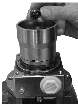
11. Mount the retainer guide on the spring guide.
