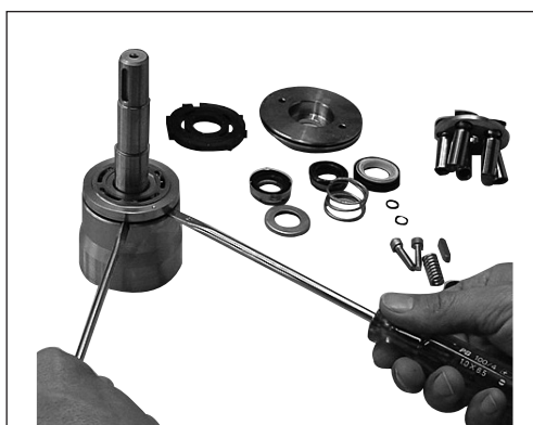
13. Loosen the valve plate using two screwdrivers. Place one of the screwdrivers in the slot of the valve plate.
