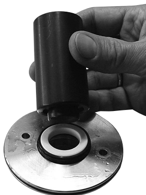
22. Wet the shaft seal with water and mount it in the front cover. Ensure that it is pressed to the bottom.
