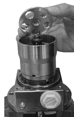
12. Mount the retainer plate on the retainer guide. Ensure that the bended surface points downwards.
