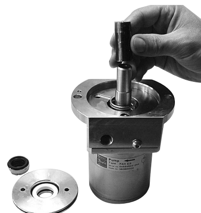
25. Fit the hollow bush onto the shaft.
